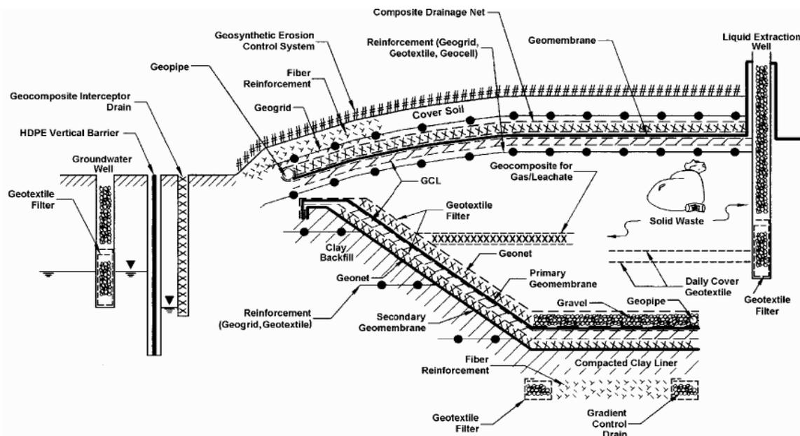
Multiple uses of geosynthetics in landfill design.
